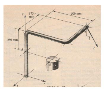
15. An 1800 N sign is supported by a 73 mm O.D. standard weight steel pipe as in the figure. The maximum horizontal wind force acting on this sign is estimated to be 400 N. Determine the state of stress caused by this loading at points A and B at the built-in end. Principal stresses are not required. Indicate results on sketches of elements cut out fom the pipe at these points. These elements are to be viewed from outside the pipe.
